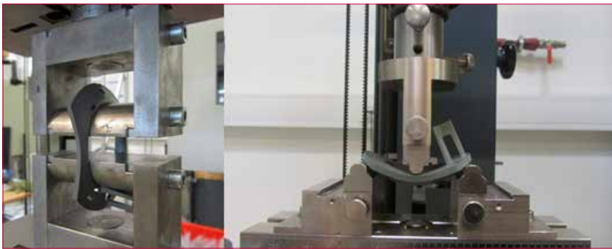
Figure 6: Component testing on the ÖkoEff clamp made of recyclate (left: ring tensile test, right: component bending test).
