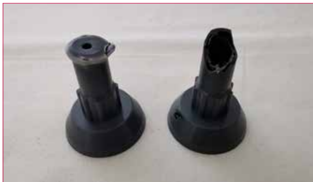
Figure 8: Nail cone after impact test at -20^{\circ}\text{C} (left: PE recyclate, right: PE recyclate with higher PP content).
