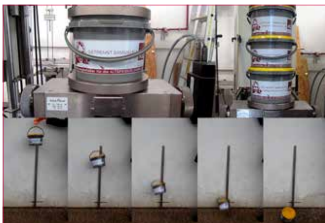
Figure 4: Examples of component tests on the bucket made of recyclate (top left: Compression test, top right: stacking compression test, bottom: Drop test on filled bucket).
