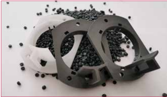
Figure 5: Examples of the ÖkoEff clamp made from virgin material (left) and recycled material.
